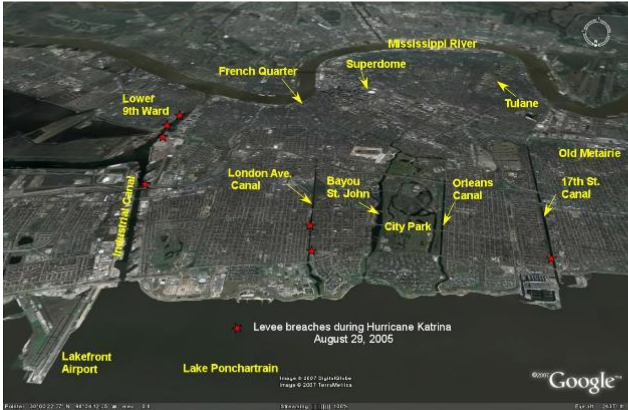
Figure 36 Levee Failure Locations – Hurricane Katrina 2005
